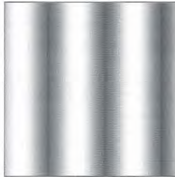
Figure 8.2 An image with a horizontal sinusoidal variation in grey level.
