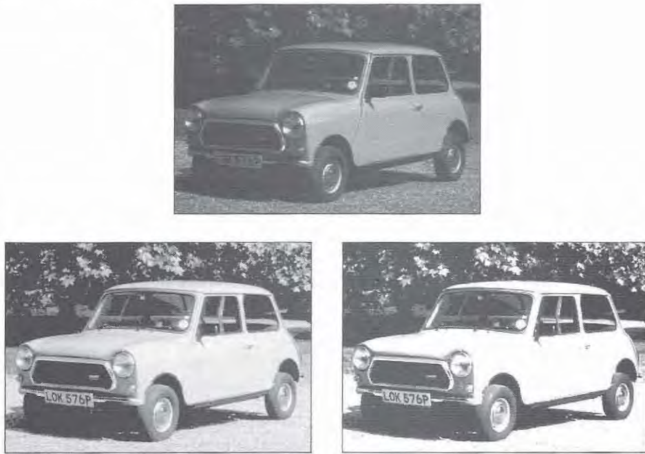
Figure 6.8 Example of logarithmic mapping. Top: an underexposed image. Bottom left: result of logarithmic mapping, making the number plate readable. Bottom right: an attempt to achieve similar results with linear mapping.
