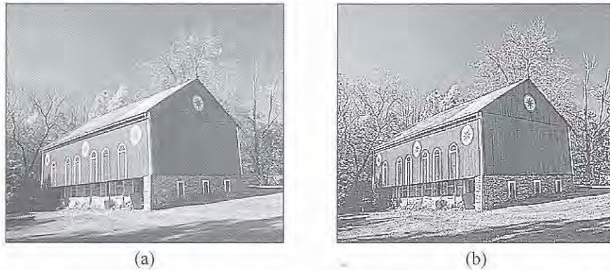
Figure 7.16 High boost filtering of the image in Figure 7.13(a). (a) Result of filtering with central coefficient c = 12 . (b) Result of filtering with c = 9 .
