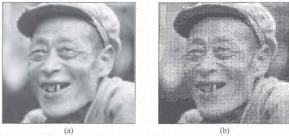
Figure 5.11 Halftoning with a binary font. (a) 8-bit greyscale image. (b) halftoned image.
