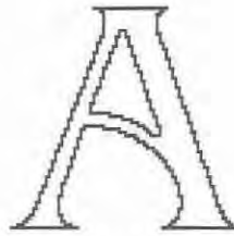
Figure 11.5 A region boundary detected by subtracting an eroded image from an uneroded image.
