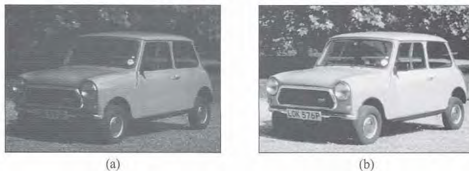
Figure 1.5 Example of contrast enhancement. (a) Image of a car with an unreadable number plate. (b) Result of contrast stretching.
