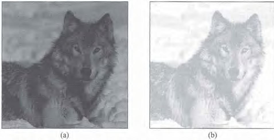
Figure 6.1 Image brightness modification. (a) A dark image. (b) Result of adding 150 to pixel values.
