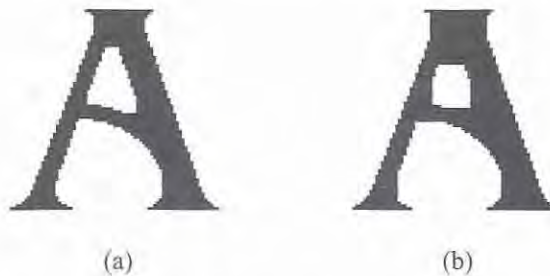
Figure 11.14 Closing of the letter A image by square structuring elements. (a) 5 \times 5 . (b) 9 \times 9 .
