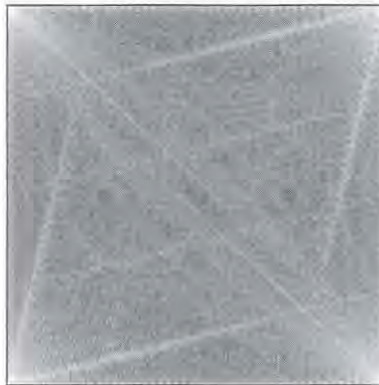
Figure 8.12 Unshifted amplitude spectrum of an image. Frequency increases from the corners towards the centre of the spectrum.
