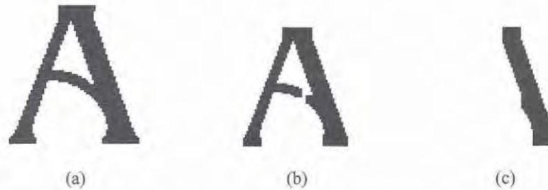
Figure 11.12 Openings of the letter A image by square structuring elements of various sizes. (a) 3 \times 3 . (b) 5 \times 5 . (c) 9 \times 9 .
