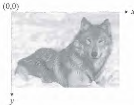
Figure 3.1 Coordinate system for an image.
